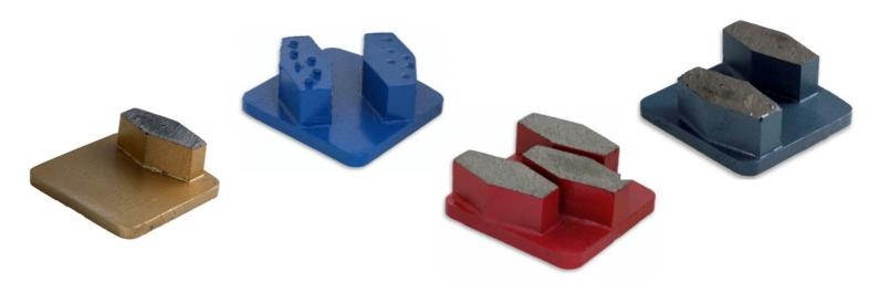
The Impact metal bond range is an outstanding diamond tool range designed to deliver incomparable high impact productivity. An excellent choice for surface preparation through to high end polishing applications where outstanding results are required. With a simplified 4 bond system covering very soft to very hard concrete the Impact segment at 6.5cm<sup>3</sup> is 20% bigger than 40x10x13mm segment and 40% bigger than 40x10x10mm segment. Money back satisfaction guarantee.
