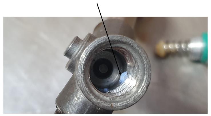
Ensure spring mounted valve seal is free from any build-up
